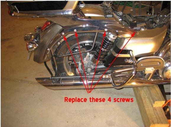
Remove the 4 bolts inside the trunk that you hand tightened earlier and replace the 4 upper side trim screws.
