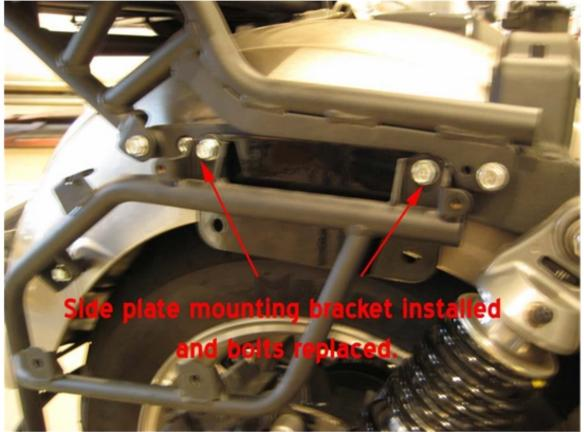
Place the side plate behind the mounting bracket and attach the side plates to the mounting brackets with the two bolts supplied with the hitch (We recommend using Loctite on this step) Repeat this step for both sides of the bike.
