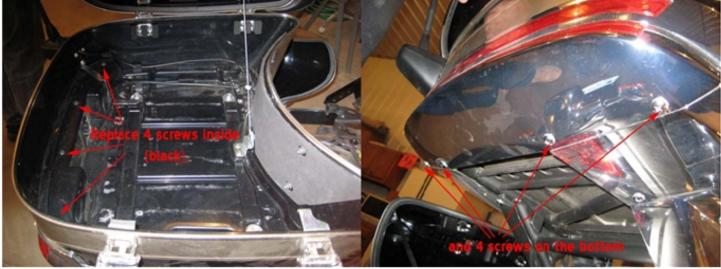
Now tighten the 4 bolts inside the trunk that you hand tightened earlier. Replace the trunk liner. Makes sure the center pins of the fasteners are pulled up, place in the hole, then gently push the center pin in until you hear or feel a slight click.
