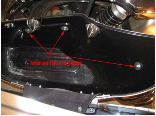
Remove the plastic liner in the bottom of the trunk by gently pushing in on the center of the plastic clips
