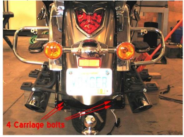
Now is the time to double check that all bolts are tight. Replace the lower piece of side trim and attach with 1 screw (Repeat for both sides of the bike).
