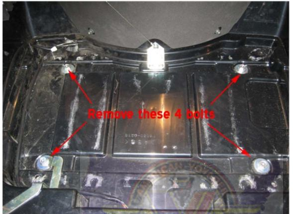
Have a friend hold the trunk up and remove the 4 screws (two on each side) for the side trim
