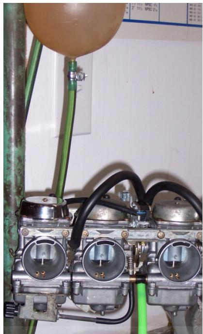
Hook up a piece of clear tubing to one of the bowls looping it back upwards as shown below.
