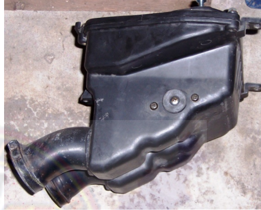
Right Side of Air Box with Plugged Port
