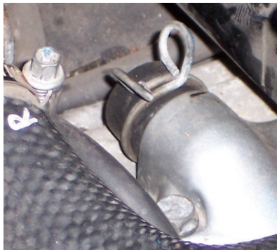
Rubber Cap on Right Suction Valve
