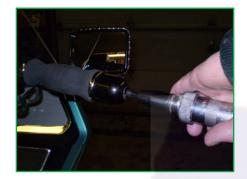
1. First, remove the stock handlebar end weights and disregard those. You will not be re-using those after the switch. The best way to remove the bar ends, is to use an impact driver with a Phillips end bit and unscrew. The bar end screws may have thread locker on them, so it may take a little persuading to get them loose and off. Shown in the picture here is the accessory Kawasaki grips which are no longer available.
