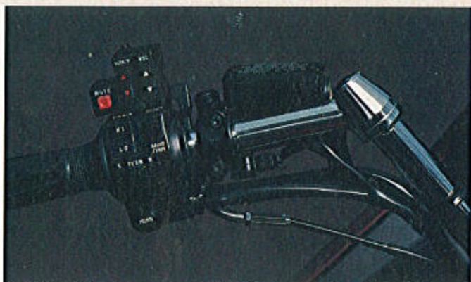
The left handlebar houses remote switches for the stereo. Large bar-end damper weights eliminate grip vibration.
