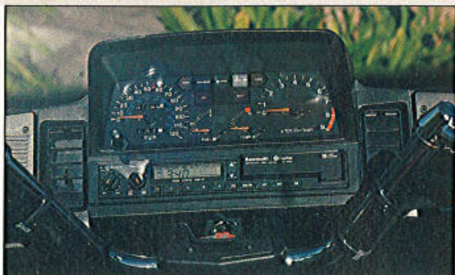
The Voyager XII's instrument panel uses easy-to-read analog gauges and convenient overdrive indicator and low fuel warning lights.
