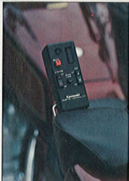
Passenger's stereo remote control, like the handlebar control, still has room for the optional CB and intercom controls.
