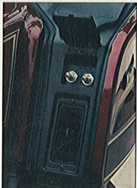
Two Schrader valves for air suspension are conveniently located beneath the cover in the right side of the fairing.
