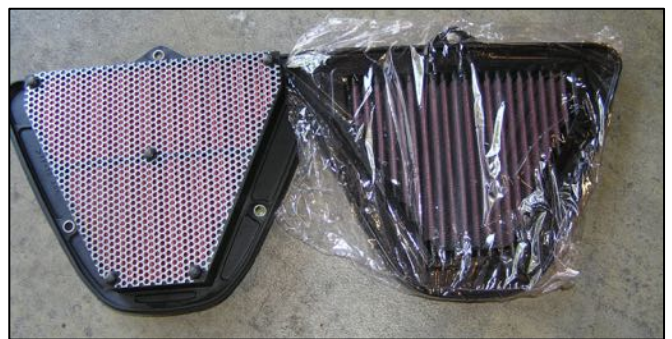
K & N air filter on the right, stock filter on left
