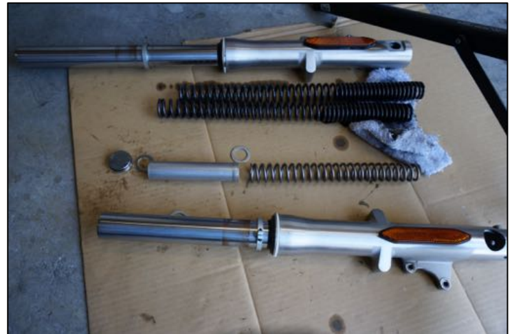
Stock fork springs on top, Race Tech fork springs on bottom
