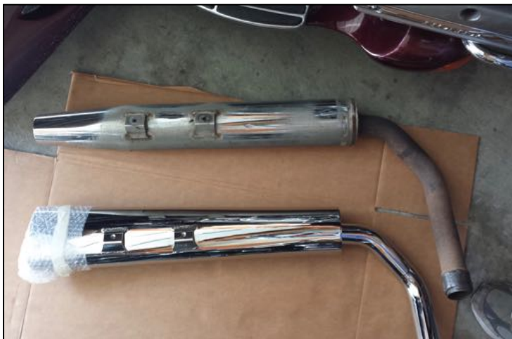
Cobra Tri-Flow muffler on bottom, stock muffler on top
