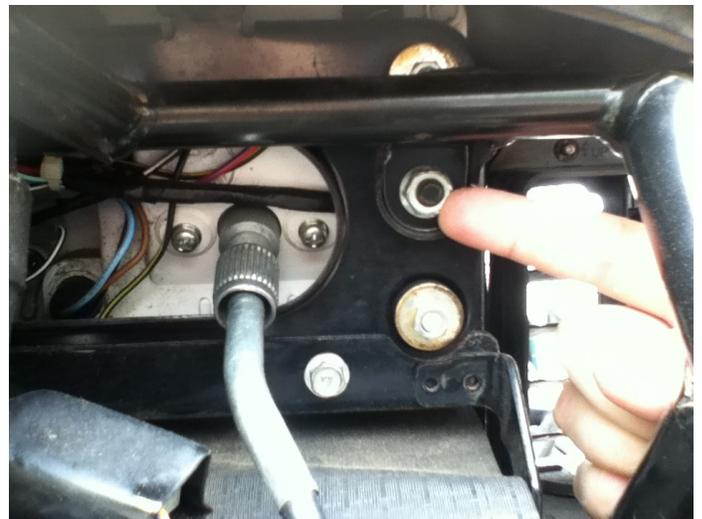
Unplug cables from the Clock cluster and the Cables from the Radio. (Power, headset, Power amp, CB. Once all unplugged, lift clock/radio cluster off the bike as a complete assembly.
