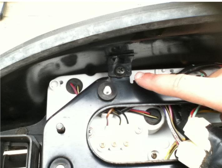
Remove the two screws holding the plastic cowl to the frame. CAREFULLY lever the upper cowl up so these pastic tabs clear the frame mount points and remove plastic cowl from the assembly.
