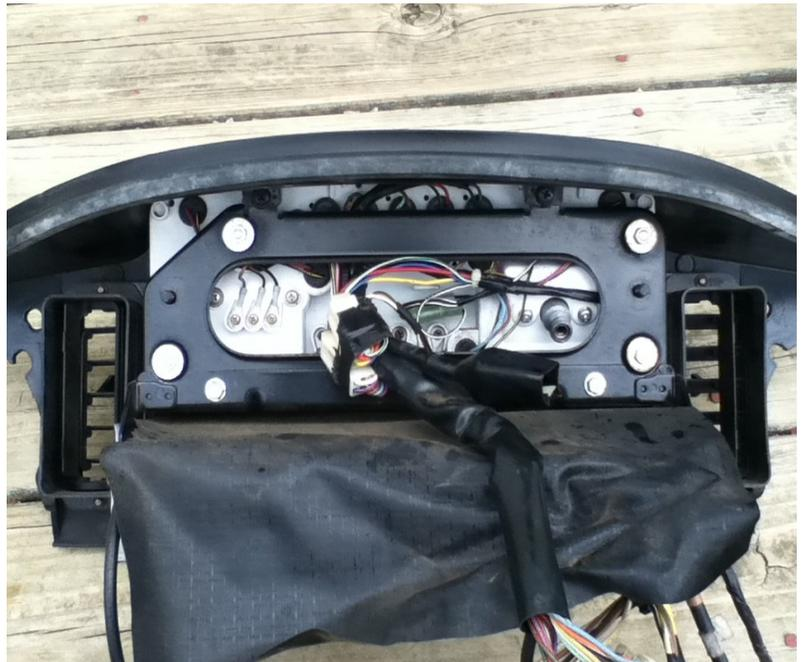
Unscrew the Vibration dampers either side of the radio. They may be perished, Keep both halves. They can be “glued” with Silicon Gasket. Remove bolts from the radio AND the frame. Remove the two screws from the bottom of the radio as shown.
