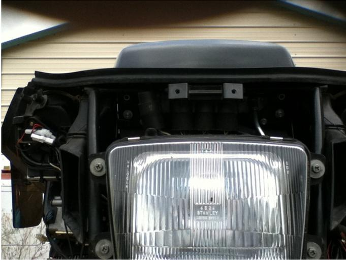
Remove Windshield, fairing uppers and lowers. Remove 4 bolts round headlight and remove and allow to dangle. With headlight moved, gently move relay clusters (4 round units above headlight).. Remove 2 10mm Bolts holding clock/radio subframe as indicated. Unscrew Speedo Cable and
