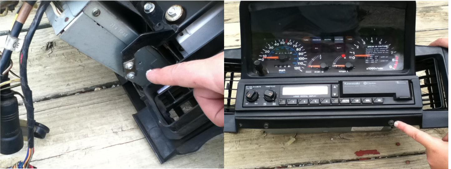
Turn assembly over and remove the 4 bolts (8mm) and washers that hold the clocks to the frame as shown below.
