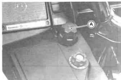
A. Headlight Vertical Adjuster
