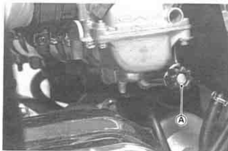
A. Idle Adjusting Screw
