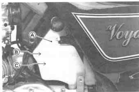
A. Reservoir Tank B. FULL Mark
