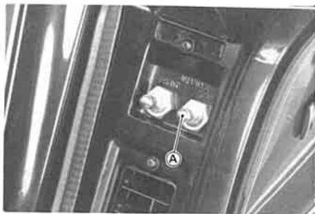
A. Rear Shock Absorber Air Valves
