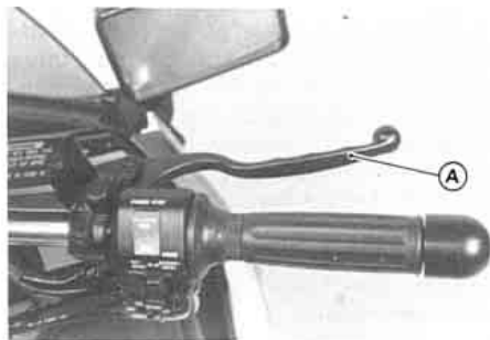
A. Front Brake Lever
