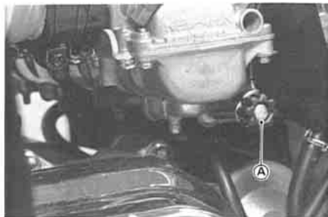
A. Idle Adjusting Screw
