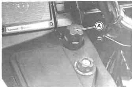
A. Headlight Vertical Adjuster
