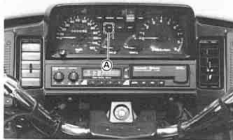
A. Oil Pressure Warning Light
